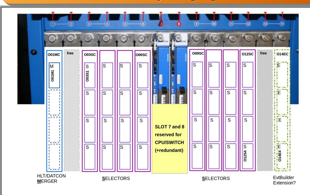
~40-45 Boards, 40-45 IPMI Boards, 42 \* locals IOCs / Run Controls
