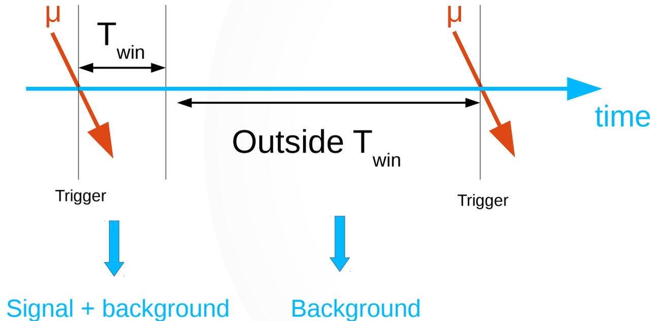
Determine the S/B ratio for different time windows (10 $\mu$ s to 50ms)
