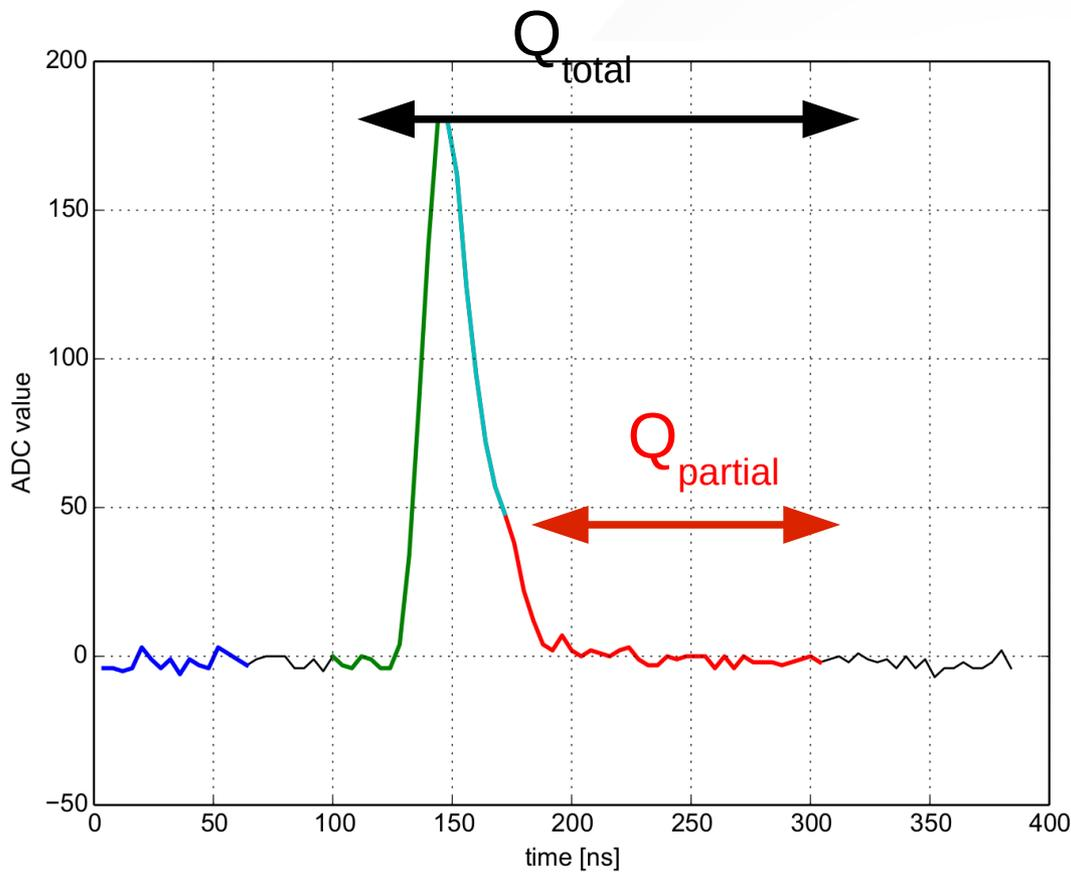
Different pulse shapes for neutrons and gammas/betas in liquid scintillator
