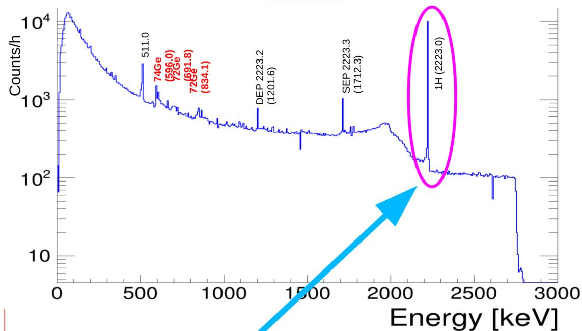
Thermal neutron capture on hydrogen with 2.223 MeV gammas
