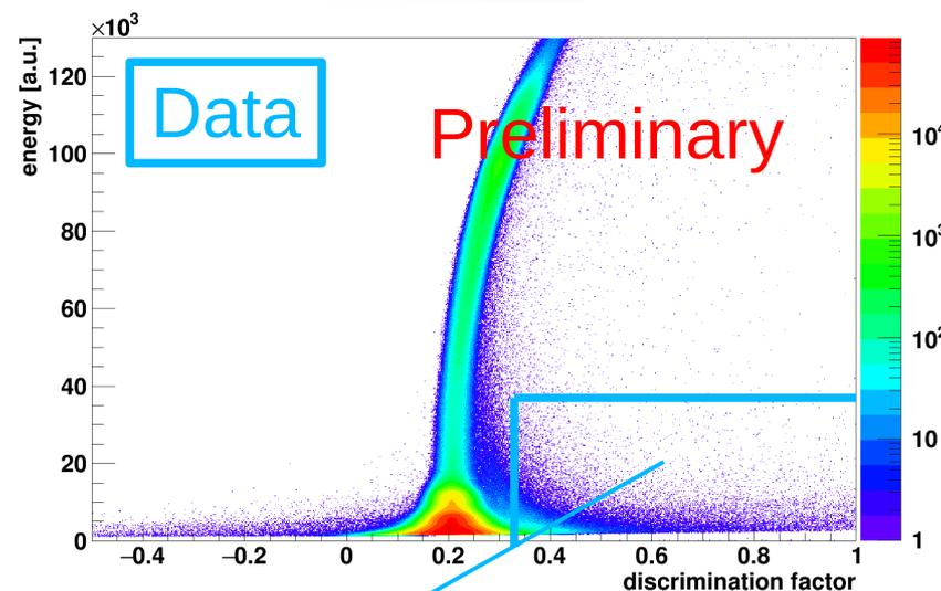
Inside time window (so after scintillation panel trigger) some orders higher neutron rate than outside time window
