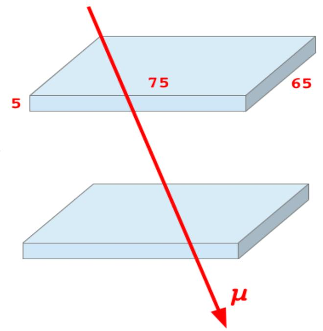
➡ Define a trigger: Allowed time difference between the panels is -40ns to +20ns
