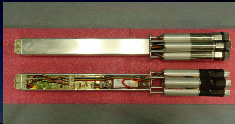
VCSEL 8kV power supply Amplifier and APD HV generator HPD Winston Cone
