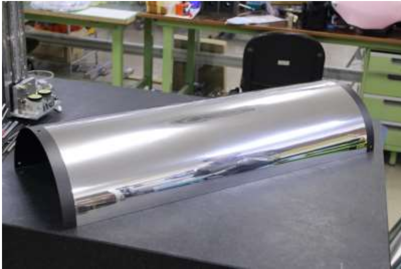
CFRP with 100umt AL sheet (grounding, shielding)
