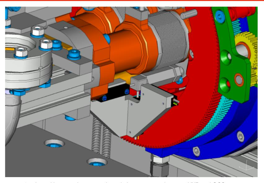
3-axis position encoders to monitor relative movement between VXD and QCS
