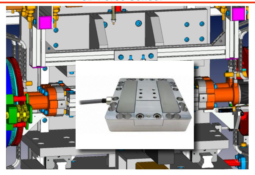
3-axis force sensor to measure resulting force on central beam pipe as function of QCS movements
