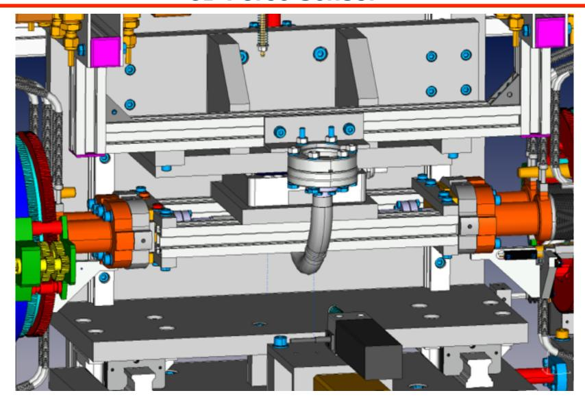
3-axis force sensor to measure resulting force on central beam pipe as function of QCS movements
