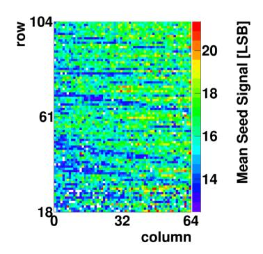
In the HV range -16V to -20V: no sign of rings for Drift -3V or -5V
