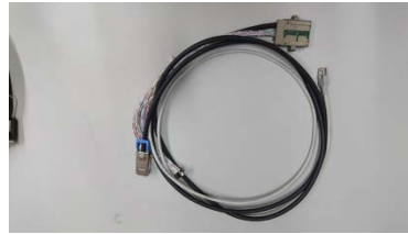
Short (2m) TWP cable with soldered PP
