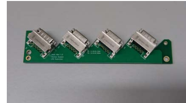
Dock box patch panel
