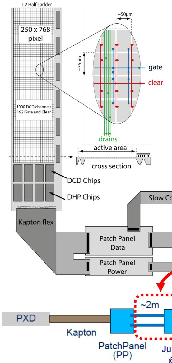
:- PXD → docks (~2m) : kapton+ Infiniband cable
