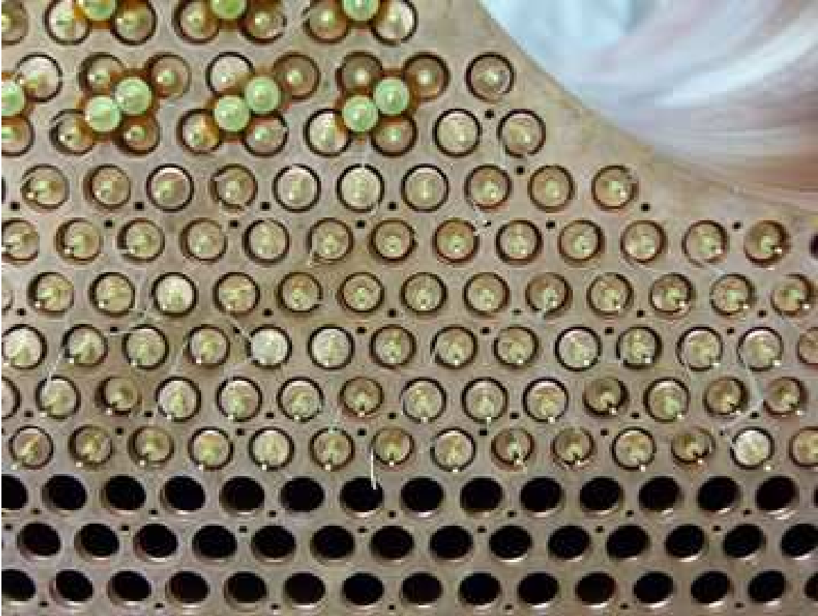
Figure 5. Photo of the front face of the FCal1 module during construction. The beam hole is partially visible in the upper right.
