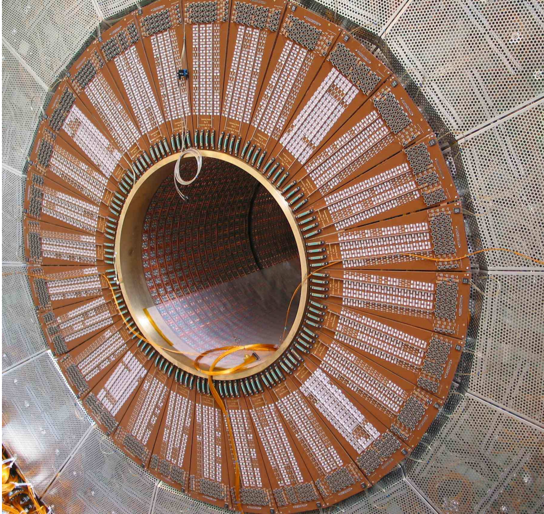
Figure 20. The 28 FCAL summing boards are mounted on the rear of the HEC calorimeter before the FCAL is inserted into the EndCap cryostat.
