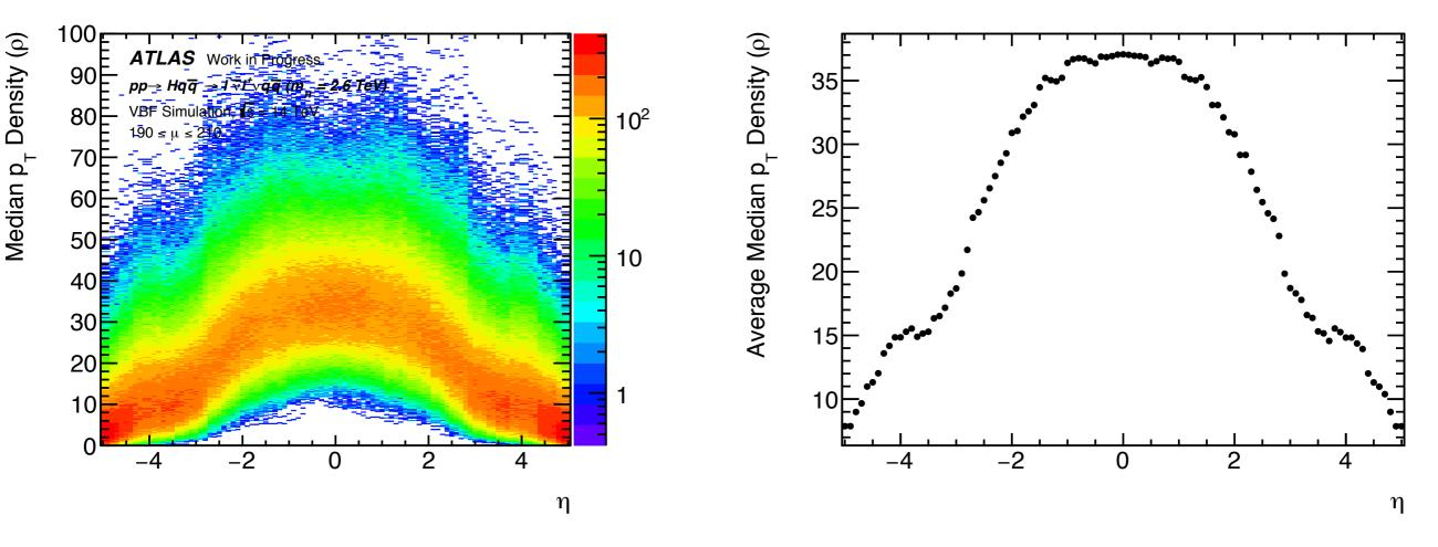
Plots above show the results of the 'SlidingWindow' approach to compute the  $p_T$  density (p) as a function of  $\eta$ . The input is **cell towers** (as opposed to LC Topo clusters).
