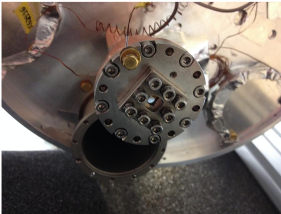
Figure : Test cell with intact window after cooldown.
