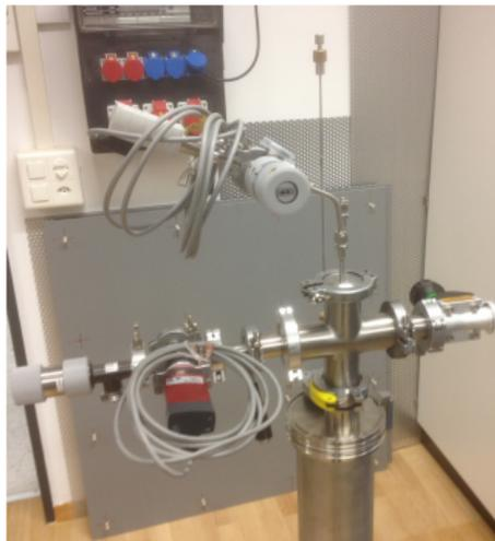
Figure : Test pipe with gauge sensors and dosing valves.
