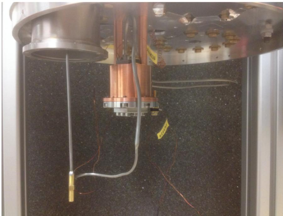
Figure : Test cell attached to the cryostat's second stage.
