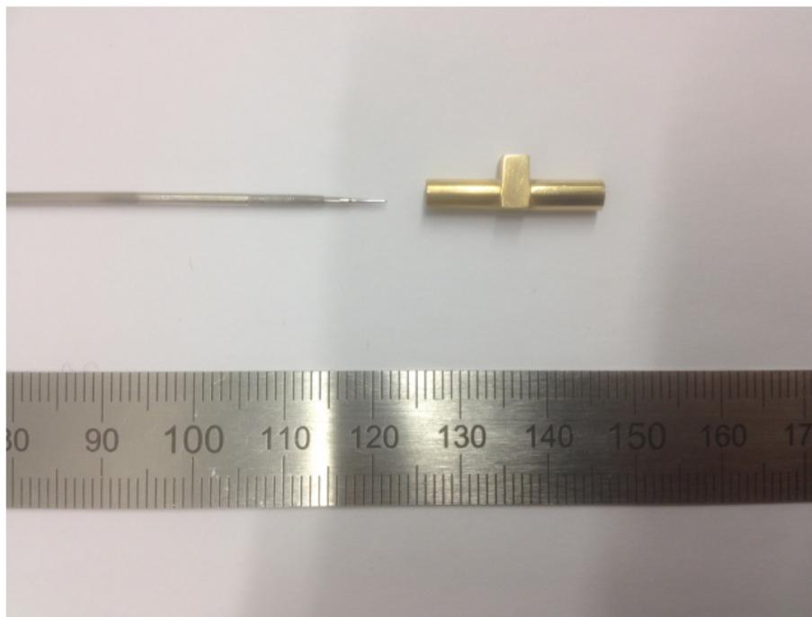
**Figure :** Custom-made cold valve (brass) with its needle (steel) to allow for differential pumping.
