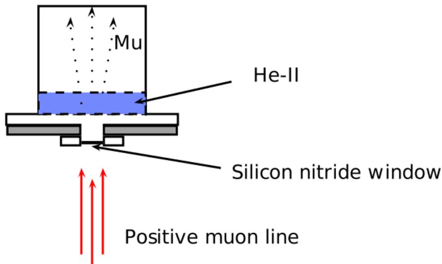
Figure : Sketch of a setup for muonium production in He-II
