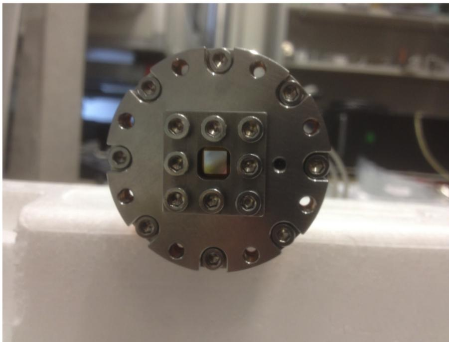
**Figure :** Indium-foil sealed,  $5 \times 5 \text{ mm}^2$  silicon nitride window for future antimuon implantation.
