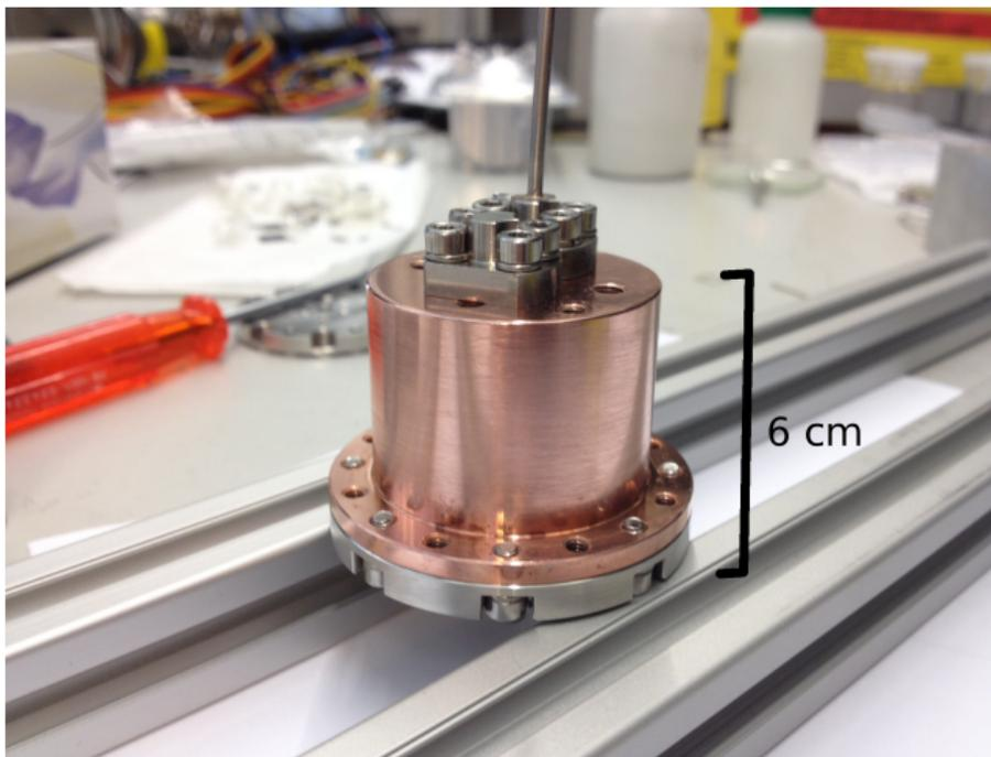
Figure : Test cell with copper container and indium-sealed steel flange.
