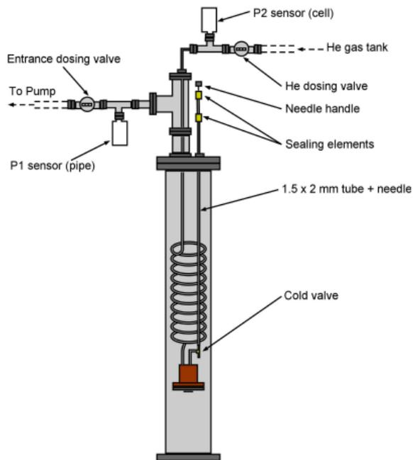
Figure : Principle: the cold valve couples the cell's inside with the outside vacuum during pumpdown.
