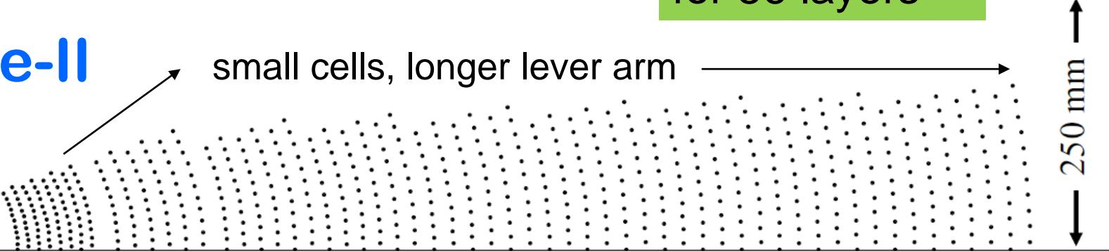
z-coordinate via standard stereo wire arrangement in 9 superlayers:
