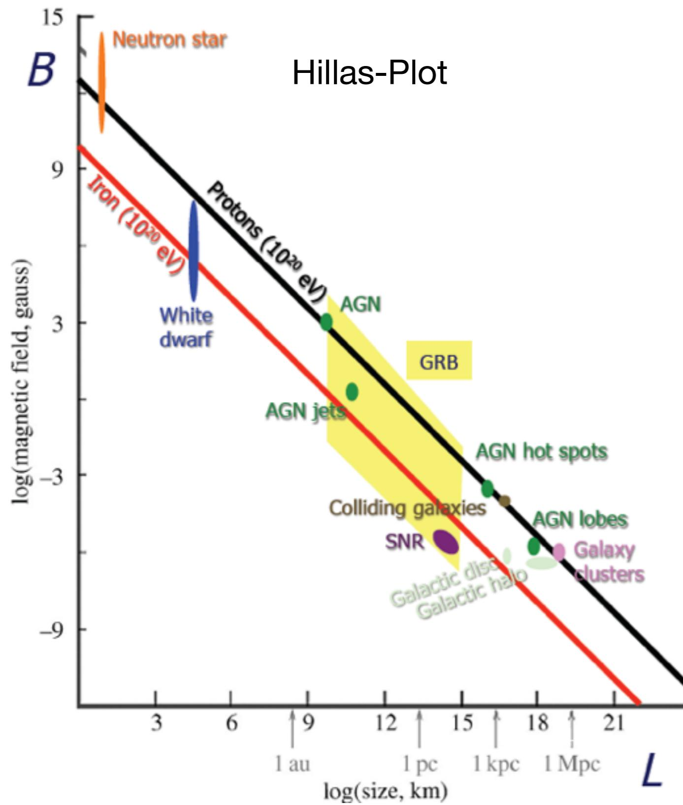
Particles are accelerated as long as they stay in the high field region:  $r_L < L$
