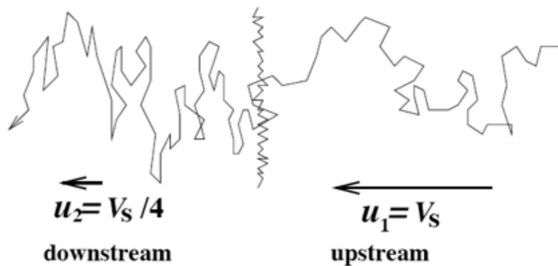
In general: the material behind the shock is 1/4 slower than the front itself, the loss rate depends on that difference:
