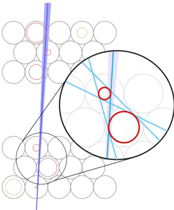
1. For every combination of two drift circles in the same multi-layer: calculate the four possible common tangents.
