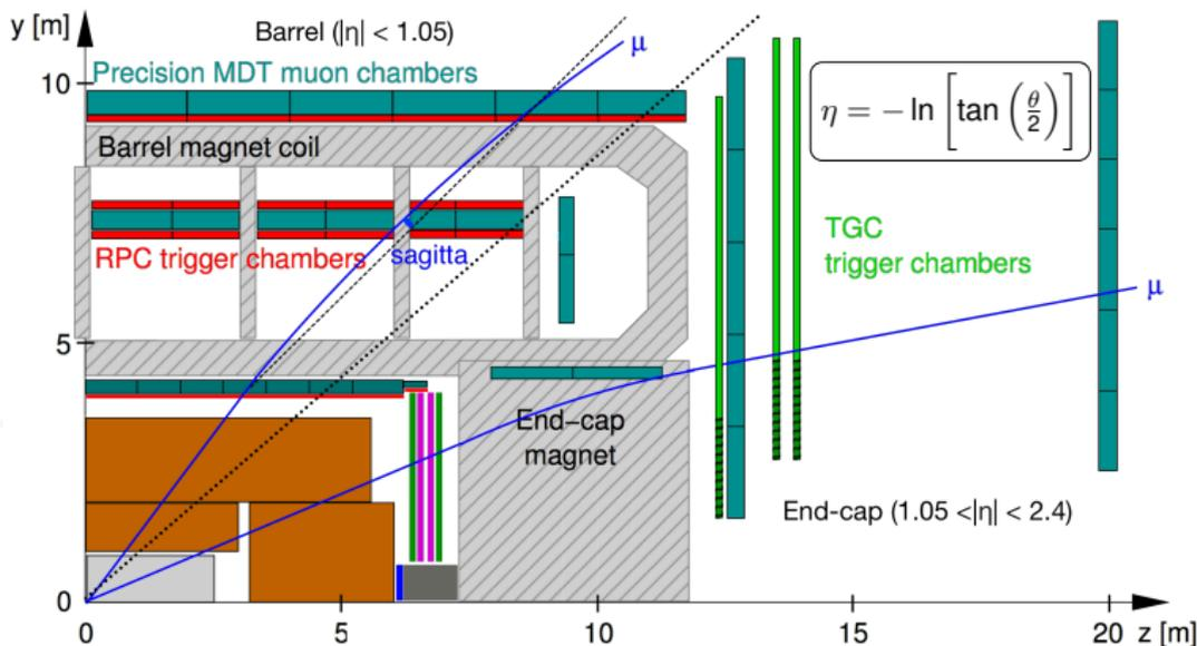
Momentum measurement from track sagitta (curvature) in three layers of muon chambers.
