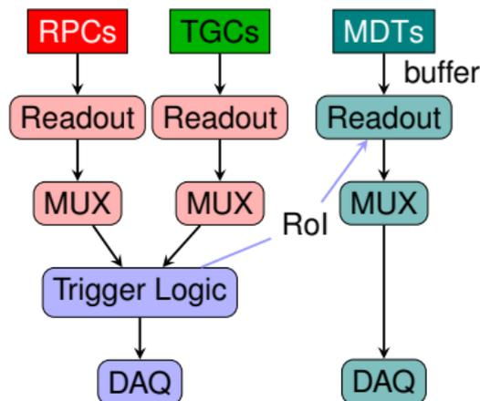
Schematic diagram of present Level-1 muon trigger
