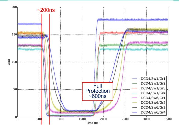
Laser Activation Timing moved forward in 10ns steps
