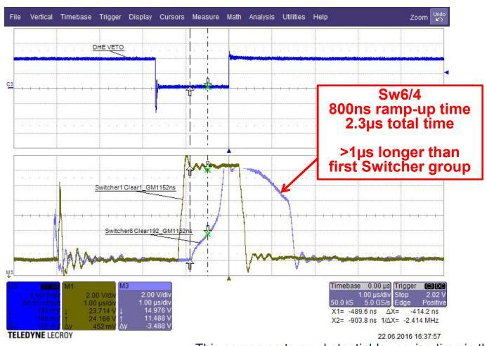
Rise time Sw1/1 ~ 200ns Rise time Sw6/4 ~ 800ns This compares to a substantial lower rise time in the SwitcherB manual but bear in mind that 6 SwitcherBs, separated into 4 groups@8Clear channels have to be switched on at once (4 times consecutively within 36 ns)
