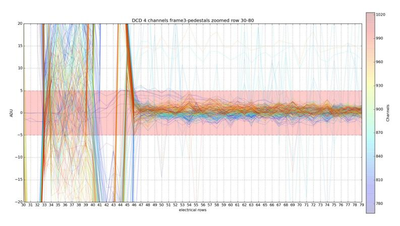
Pedestal oscillations are within arbitrarily chosen threshold limit of  $\pm 5$  ADUs not before 23 gate periods = 2,94 $\mu$ s
