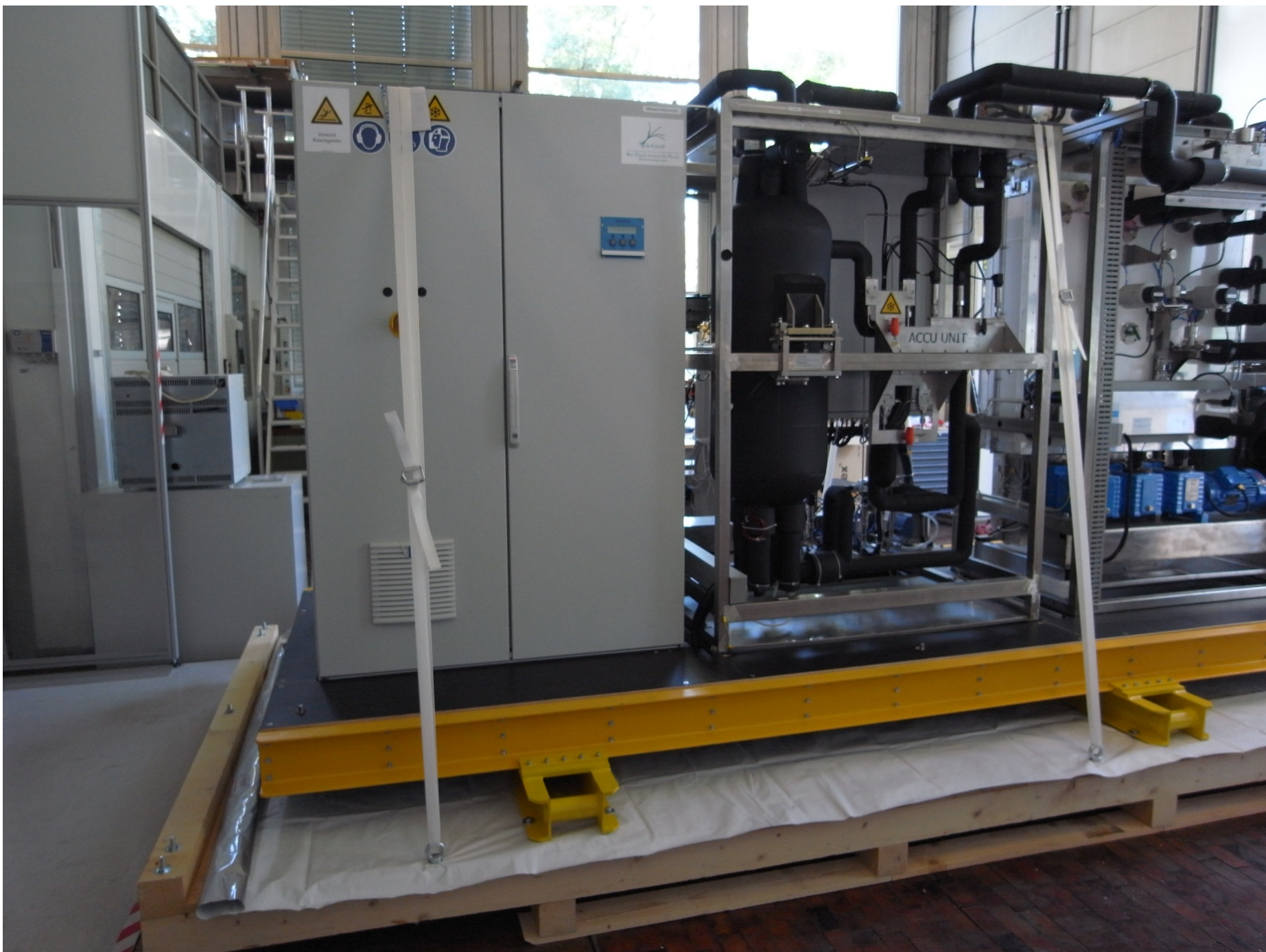
IBBelle on the pallet, secured by belts and screws. Note the water proof foil under IBBelle
