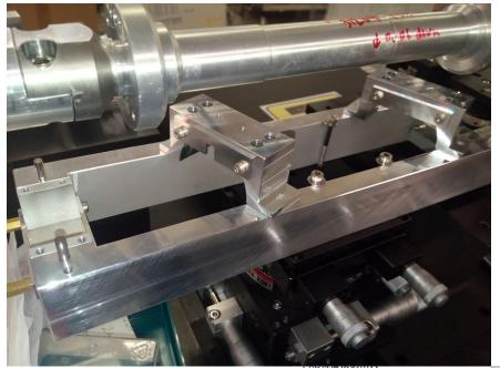
PXD mount block Alignment tool has prepared (controlling xyz position)
