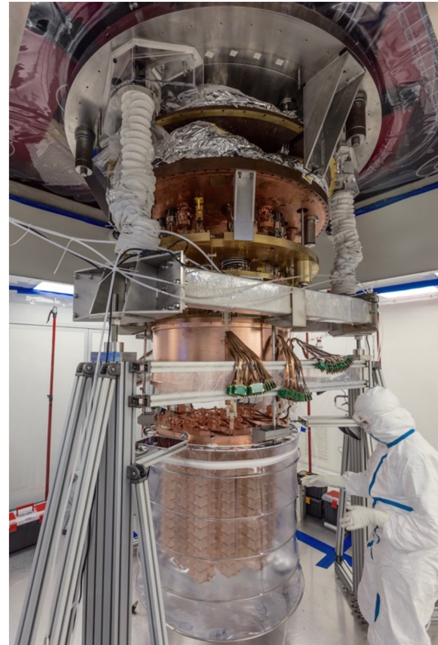
Detector stored in N 2 atmosphere
