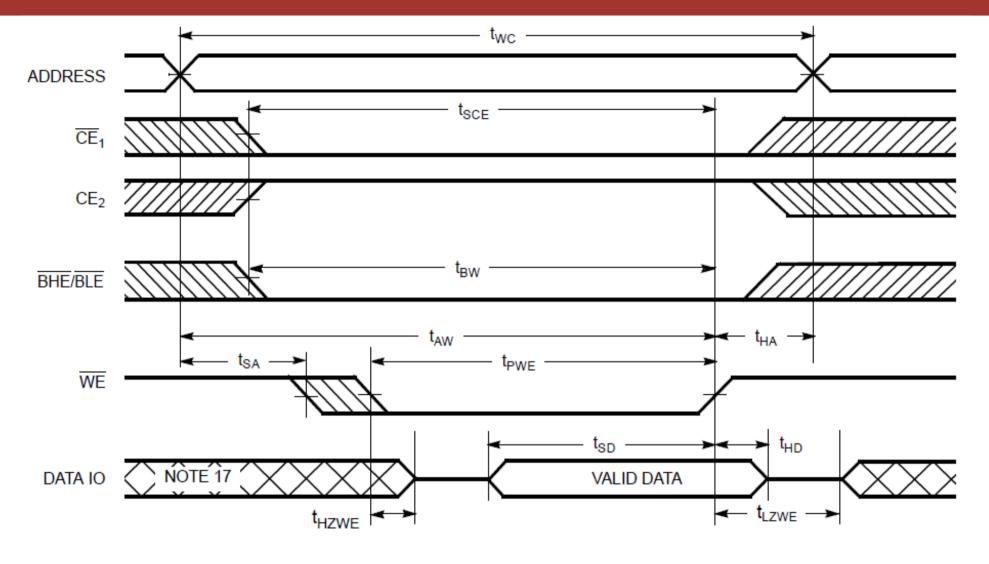
Min values:  $t_{WC}$  10ns,  $t_{SCE}$  7ns,  $t_{AW}$  7ns,  $t_{HA}$  0ns,  $t_{SA}$  0ns,  $t_{PWE}$  7ns,  $t_{SD}$  5.5ns,  $t_{HD}$  0ns,  $t_{LZWE}$  3ns,  $t_{BW}$  7ns
