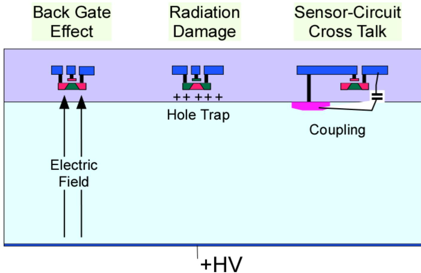
Problems: transistor operation affected by back-gate effect, signal cross-talk and charge trapped in Oxide.
