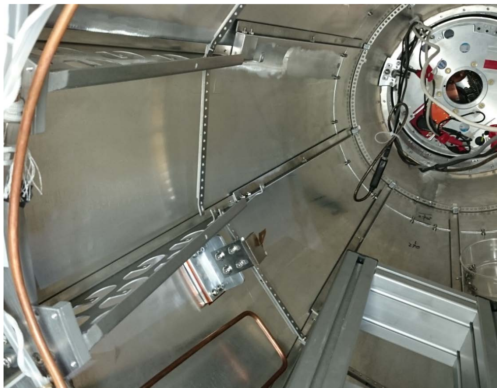
FWD CDC cable cage installed (inner spokes removed for B-Field Mapper installation)
