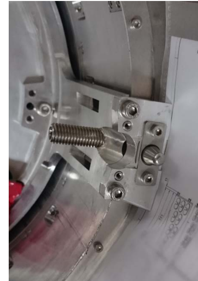
Clearance check VXD-bracket FWD-right
