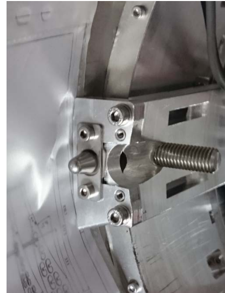
Clearance check VXD-bracket FWD-left
