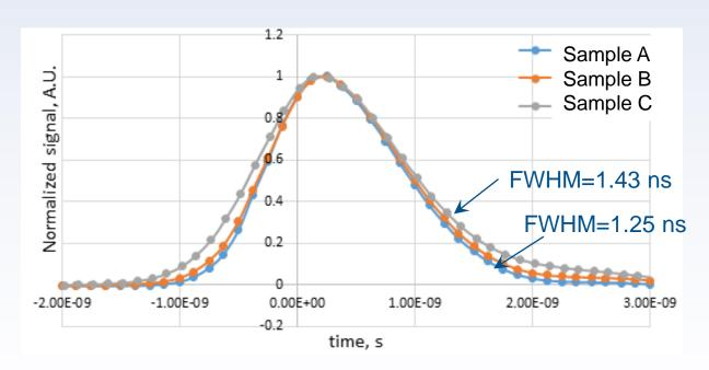
► PMT9880 FWHM: 1.2 ns → Time resolution limited by PMT response
