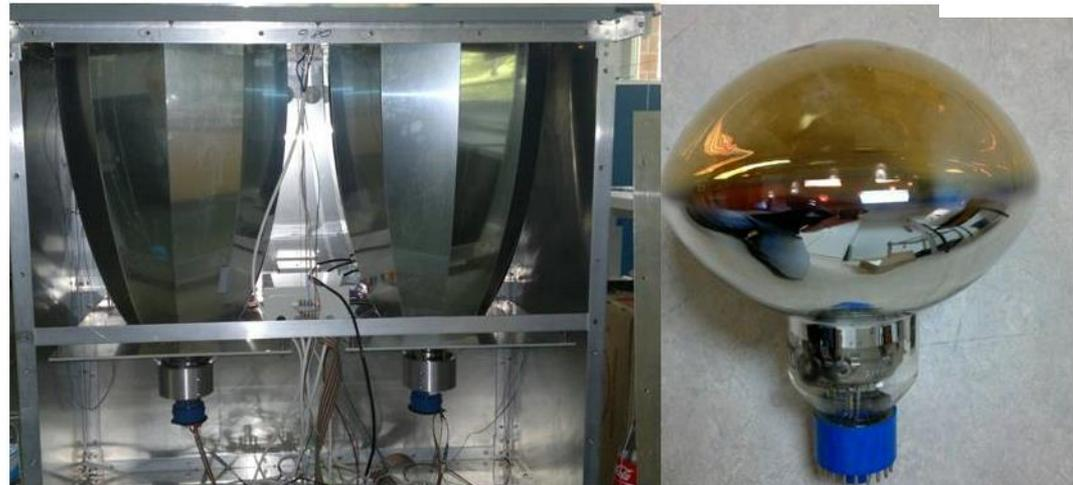
Photos of the optical station of TUNKA-HiSCORE and PMT R5912-TUNKA
