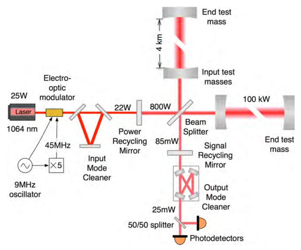
All of the components shown, except the laser and phase modulator, are mounted in the LIGO ultra-high vacuum system on seismically isolated platforms. Power levels at ca. 1/8 of design values.
