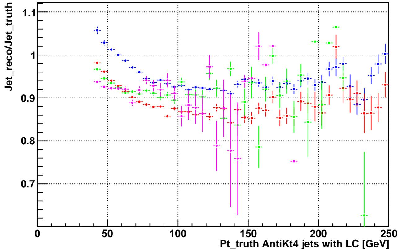
Jets linearity distributions obtained with AntiKt LC jets. Blue (red) distribution is for the first (second) btagged jets, green (magenta) distribution is for the first (second) selected light jets. in these plots the  $P_{\perp}^{\text{reco}} > 20\text{GeV}$ , and  $P_{\perp}^{\text{truth}} > 40\text{GeV}$
