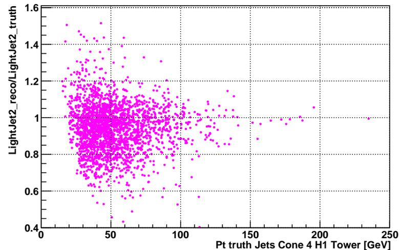
Distributions obtained with Cone4H1Tower jets. The bias introduced by the  $P_{\perp}$  cut (40 GeV and 20 GeV) to the reco jets is clearly visible. Top left (right) first (second) btagged jet, bottom left (right) first (second) selected light jet
