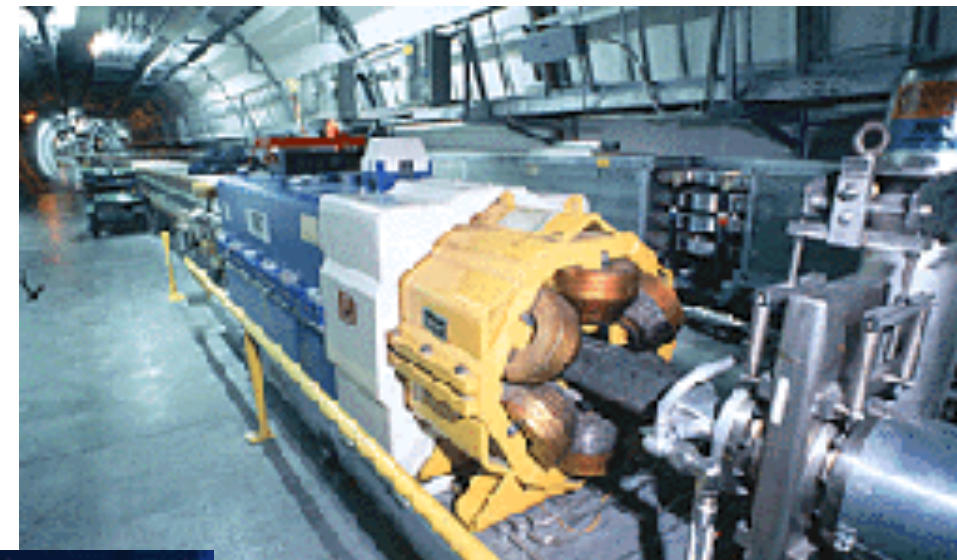
Sextupole for higher order focusing, additional beam line elements: beam pipe, pumps, ...
