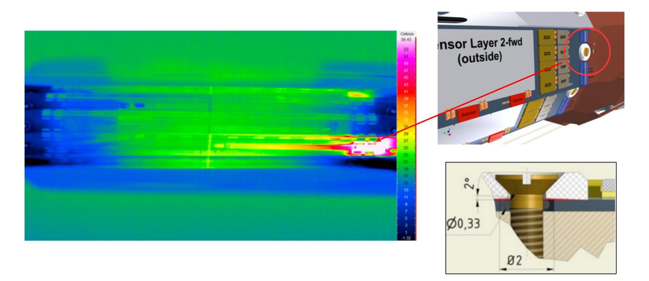
Several hot ASICs are found, due to loosen screws or blocked holes, should be tested before mounting sensors.
