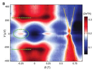
and *B*. The ZBP is highlighted by a dashed oval; green dashed lines indicate the gap edges. At ~0.6 T, a non-Majorana state is crossing zero bias with a slope equal to ~3 meV/T (indicated by sloped yellow dotted lines). Traces in
