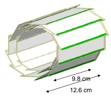
Small, thin (50µm) Detector: 2 layers, 20 modules (in total)
