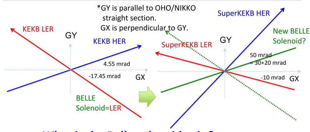
What is the Belle solenoid axis? Solenoid axis is:
