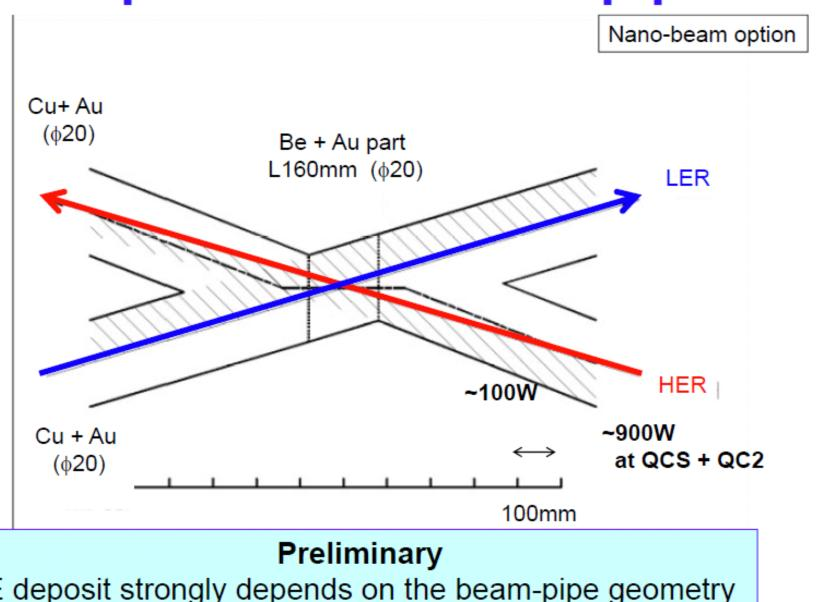
E deposit strongly depends on the beam-pipe geometry
