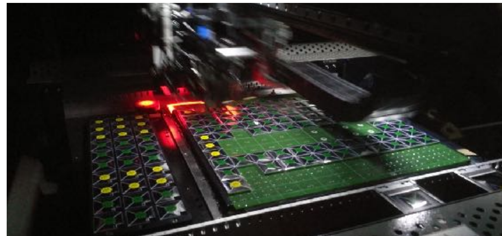
semi-automatic wrapping of 22k scintillator tiles
