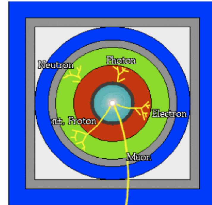
**Tracker:** Momentum of charged particles via deflection in magnetic field and precise track reconstruction
