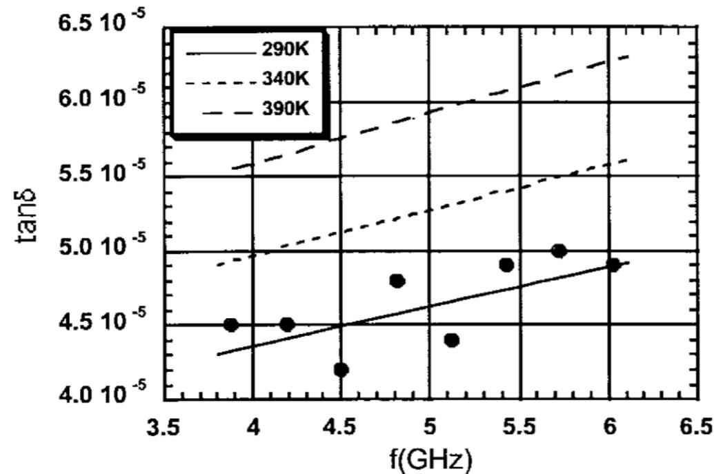
Fig. 6. Results of dielectric loss tangent measurements versus frequency for low-loss ceramic as determined with whispering-gallery-mode dielectric resonator technique.
