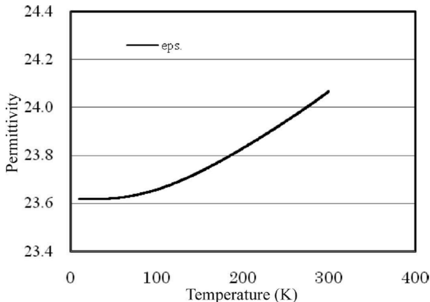
Fig. 2. Temperature dependence of permittivity of  $\text{LaAlO}_3$ .
