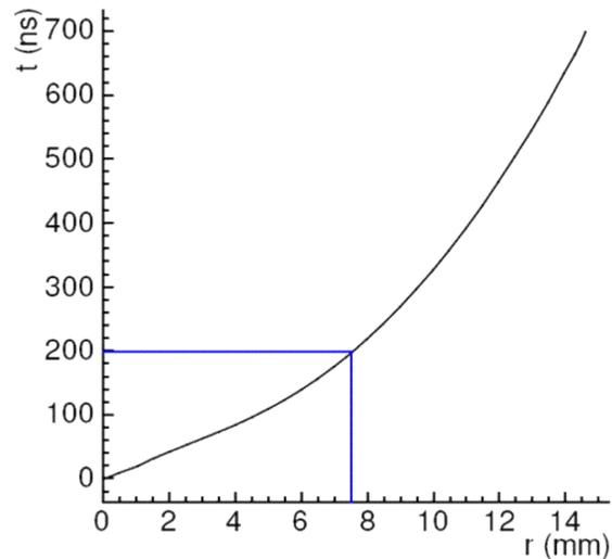
By reducing the tube diameter from 30 to 15 mm we get a shorter maximal drift time and a more linear space drift time relation
