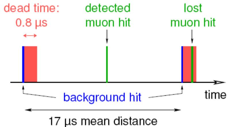
Some muon hits are masked by background events. But the track reconstruction efficiency is still good ( $\approx 90\%$ ) up to an occupancy of 30% because of the redundant measurement by 6 tube layers.
