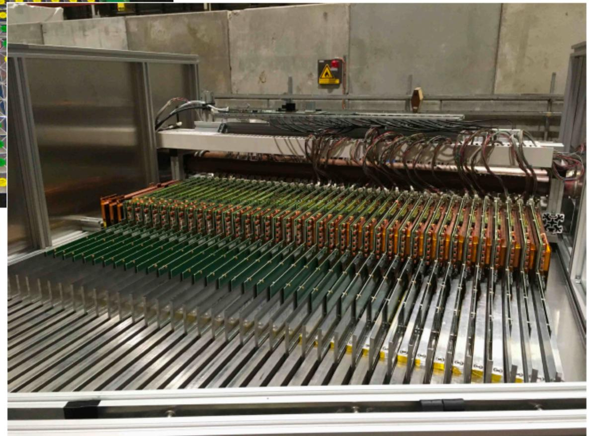
CALICE highly granular analog hadronic calorimeter (AHCAL)
