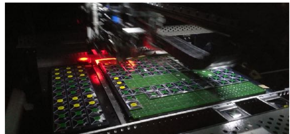
automatic mounting of scintillator tiles on electronics boards (160 boards)
