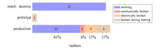
Only the "mechanically" or "electrically broken" categories are directly correlated to the gluing process. Subtracting the modules, which broke during testing, the yield of the production gluing process was at 78%.
