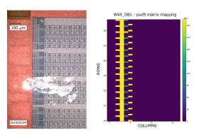
The damaged matrix of W44\_OF1 after gluing of ladder L2\_024 is shown on the left side. The bright spot is the broken BCB passivation layer. The metal lines underneath were damaged as well resulting in short-circuits. The readout of the turned off matrix on the right side shows high current in the affected drains.
