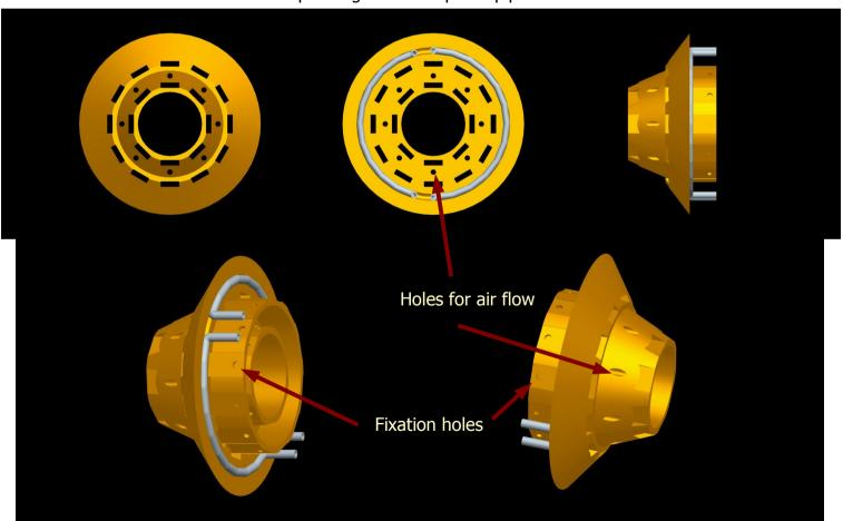
Cooling at the top allows to have air flow between the 2 layers
