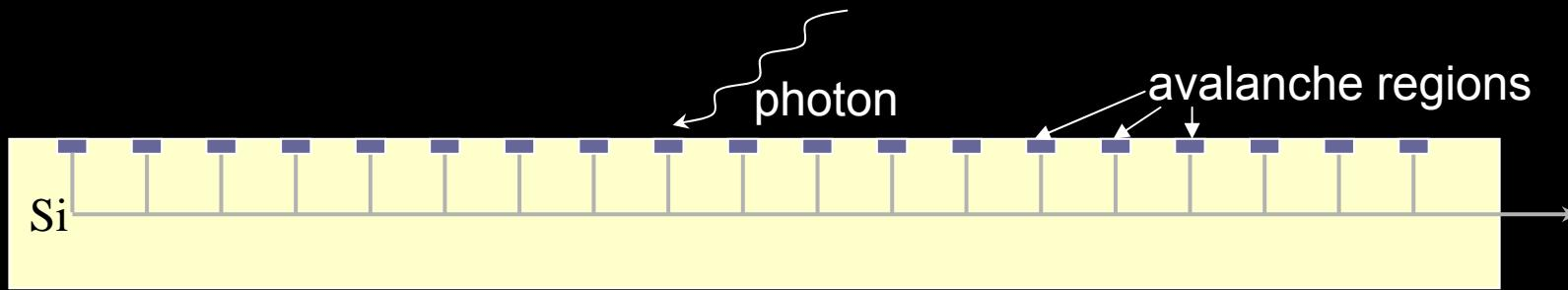
BID SiPM – combined principle of avalanche photodiode and drift diode
