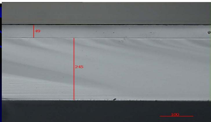
d) deep etching opens "windows" in handle wafer
