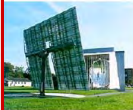
The solar concentrator at PSI and the detector assembly mounted in the focal plane.
