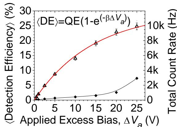
Passive quenching (PQ) failure at high biases
