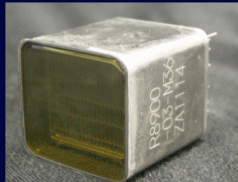
Hamamatsu R8900U-08-M36-MOD 1 inch 36ch UBA MAPMT (with 3mm x 3mm slit)
