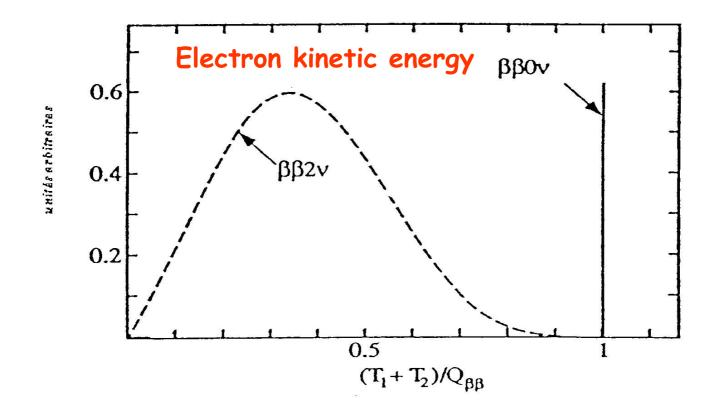
The measurement is conceptually simple - we look for a sharp peak at the end of the two-electron energy spectrum. Biggest issue is background. Need to reduce background in the energy range of interest to 10<sup>-3</sup> event/kg/year !
