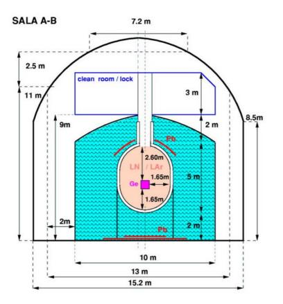
Liquid Nitrogen can be purified such that there are ~no dangerous isotopes. Nitrogen acts as shield against radiation from walls, containment vessel. Possibility to use Argon instead of Nitrogen. Switch to water for outside layer to make cryogenic vessel more compact. Water acts as Muon Veto.
