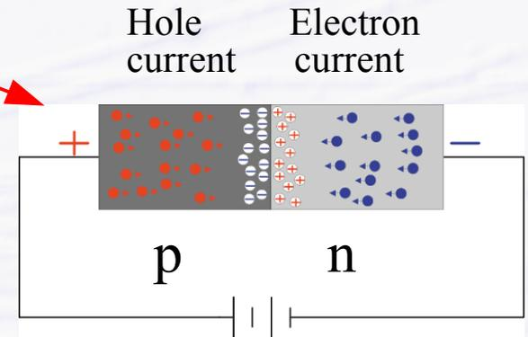
→ for use as particle detector diode needs to be connected in opposite way
