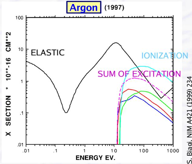
consequence: UV photons (>11.6 eV) hit surface of metals (cathode) and free new electrons, ionization energy of Cu = 7.7 eV
