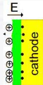
**Cathode:** ions on top of insulating layer cannot recombine
