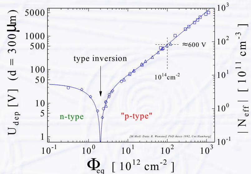
“Type inversion”: n-type material changes to p-type material after a certain accumulated radiation dose
