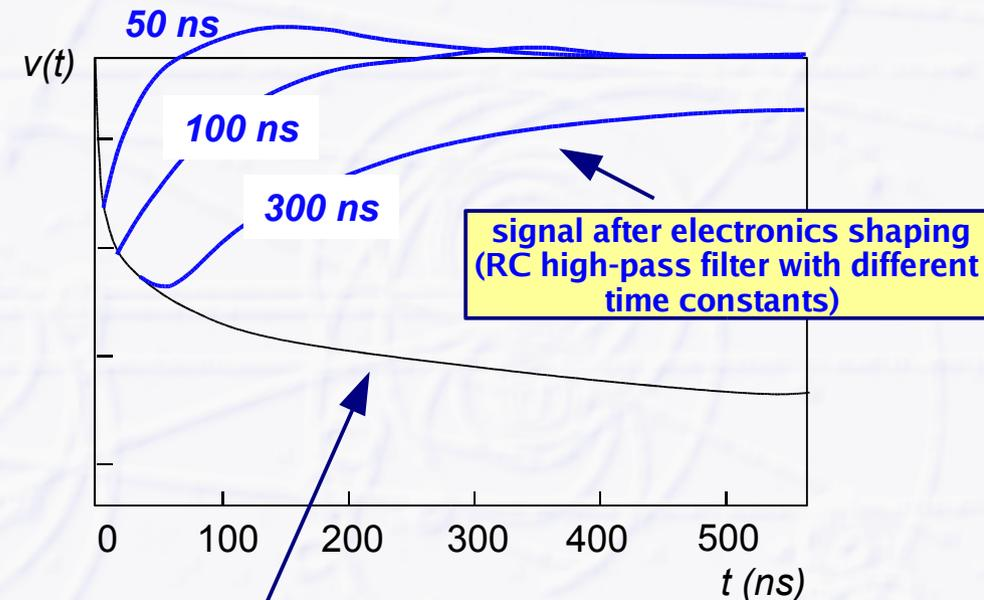
pure signal (no electronics shaping)
