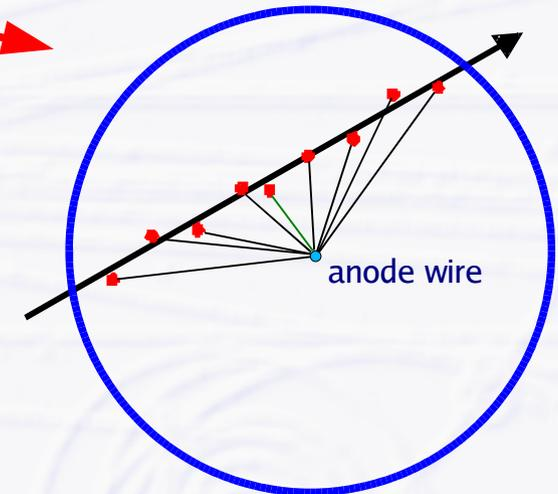
very different drift lengths of electrons for tracks close to the wire, position of fastest electron very much dependent on ionization fluctuations
