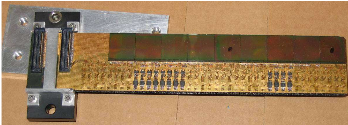
Prototype with Cu conductor and several MIMOSA-5 chips mounted
