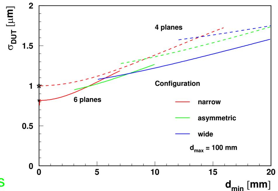
The optimum telescope setup depends on the assumed parameters.
