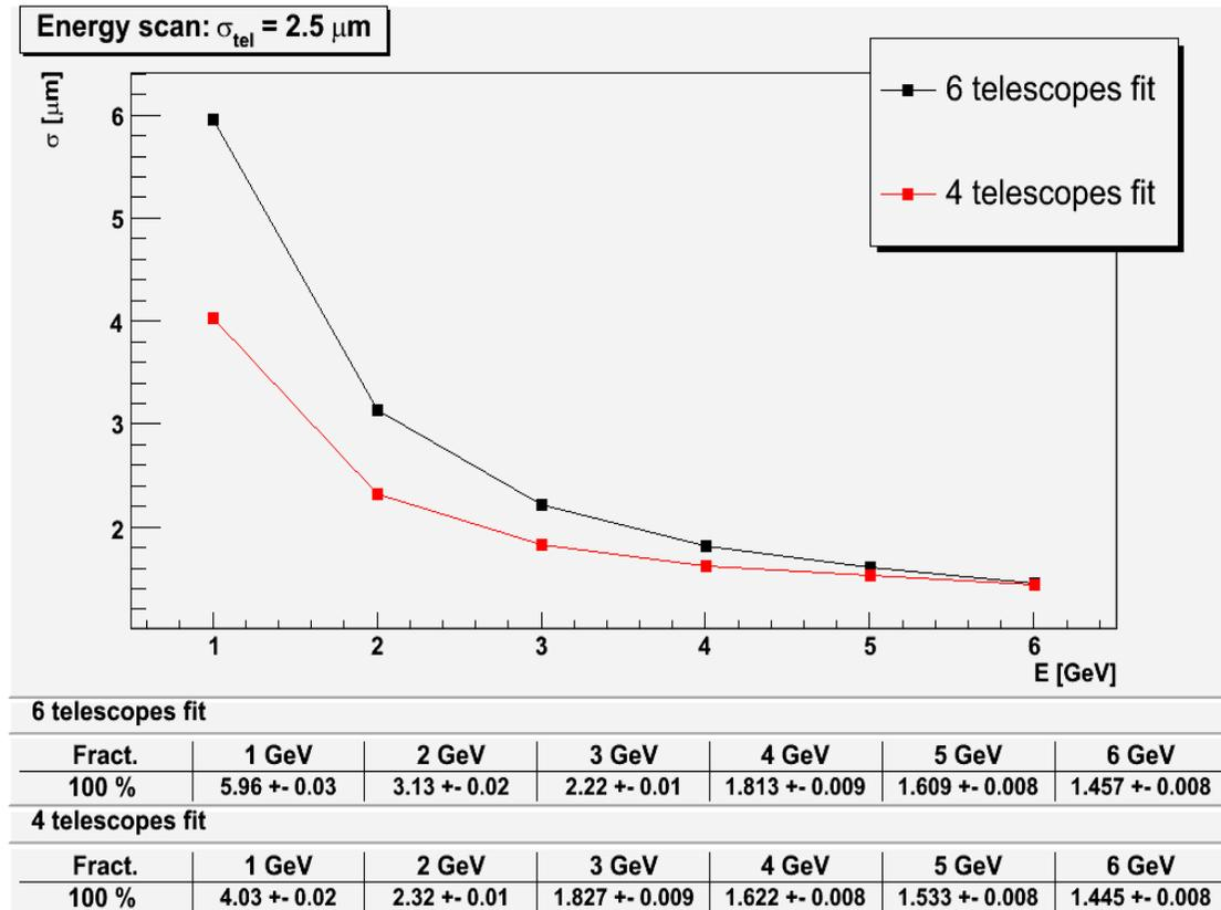
Telescope resolution  $\sim 1.5 \mu\text{m}$  at 6 GeV
