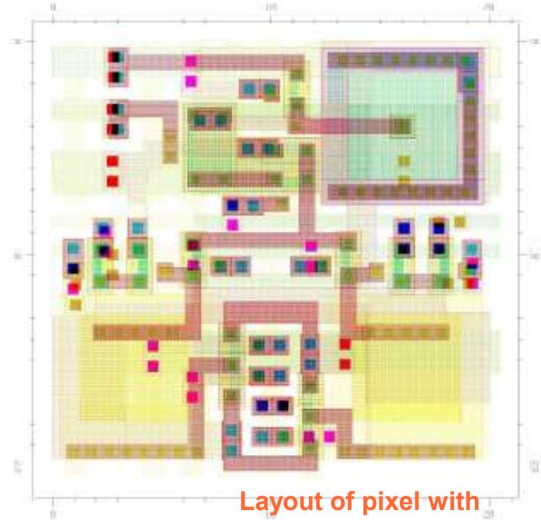
Layout of pixel with integrated CDS,  $20 \times 20 \mu\text{m}^2$
