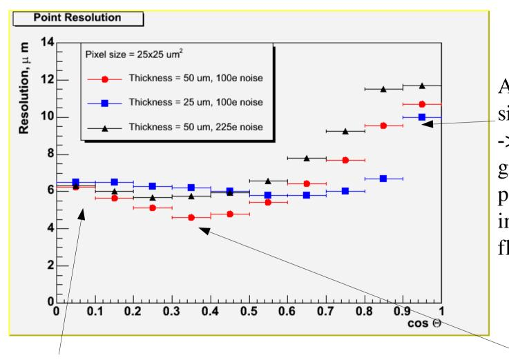
At shallow angles cluster size gets extremely large -> simple centre-of-gravity approach yeilds poor resolution due to inter-pixel charge fluctuations
