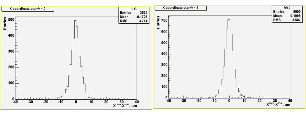
R-Phi resolution slightly improves at smaller incident angles at smaller polar angles. Explanation: longer track length within active layer -> larger deposited charge -> smaller fluctuations.
