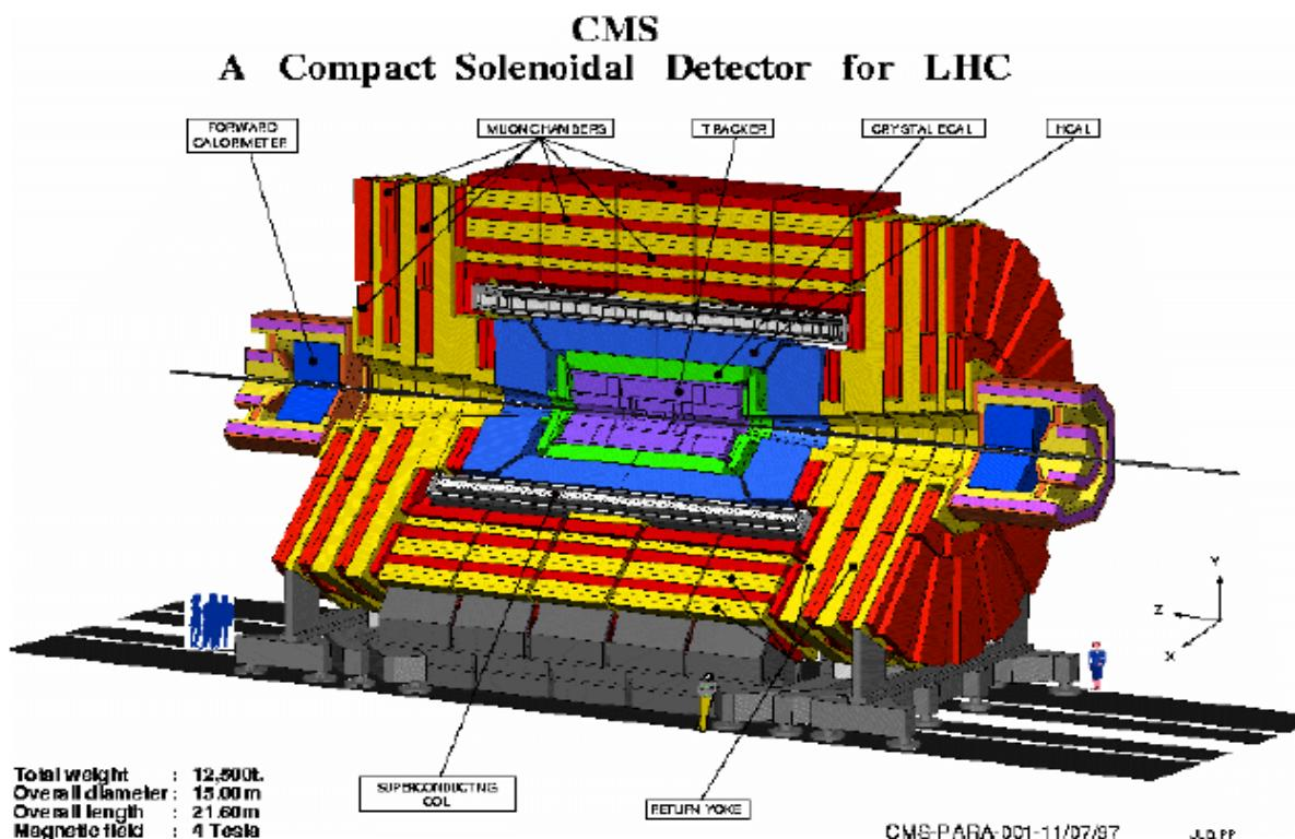
Technique: Calorimeter **inside coil**
