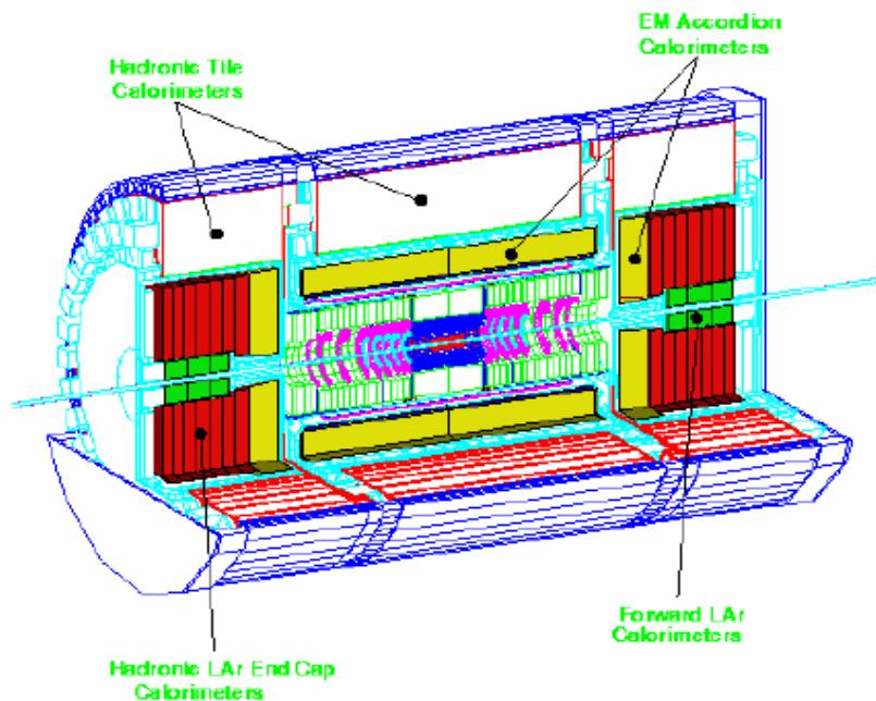
Tile–calorimeter: hadron detection
